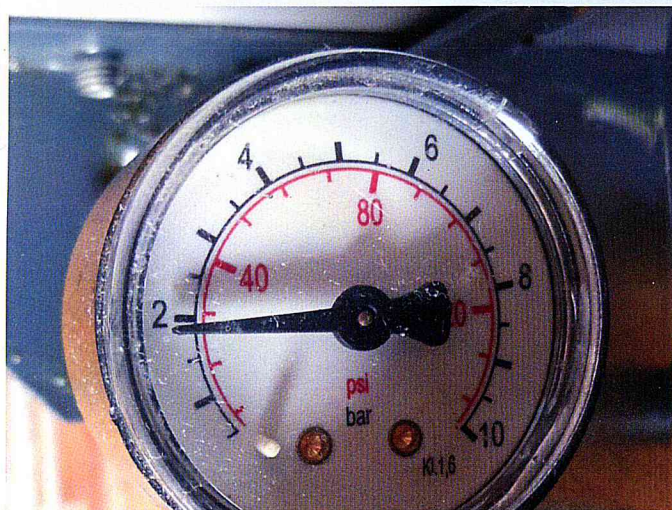
01 When using an airbrush, the pressure on the compressor must be 1.8 – 2 Bar.
