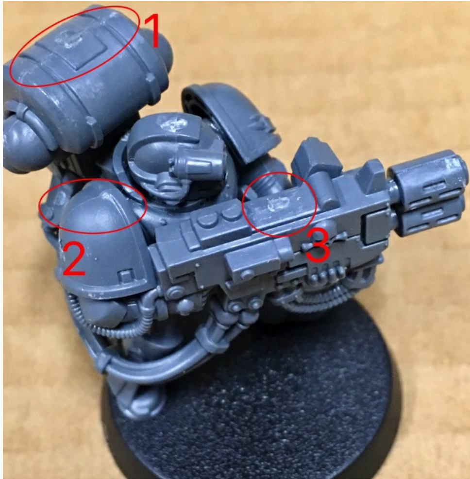
1. A seam between two pieces 2. A mold line 3. A sprue residue
